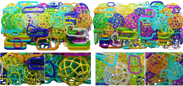
Fig. 10. Left: Locks packed without interlock checking, notice significant number of interlocked parts as highlighted on the bottom. Right: Locks packed with interlock checking, notice parts are free of interlocking, as highlighted on the bottom.
