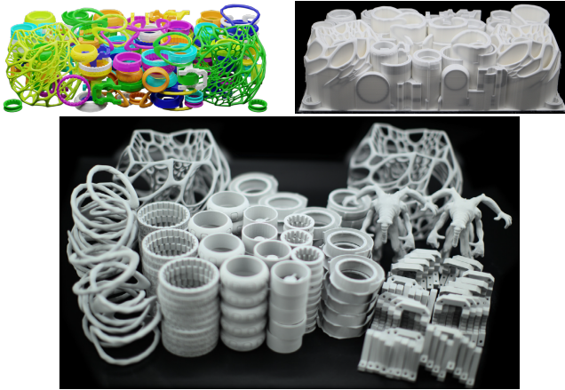
Fig. 21. Top left: The same set of objects in Fig. 20 are packed with our algorithm with no interlocking. Top right: The printed tray containing the set of objects on the left. Bottom: The disassembled printed objects.
